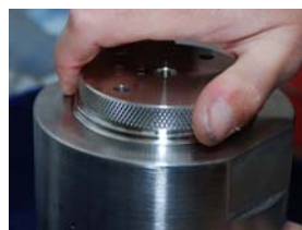
Cover screws onto vessel.
