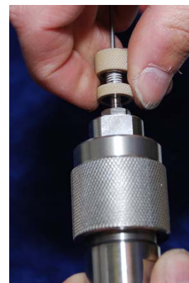
Vessel connector attaches to male fitting in end cap on assembled vessel.
