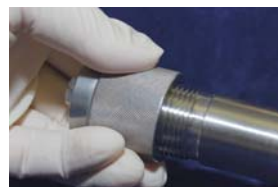
Closure nut finger tightens onto end of vessel.
