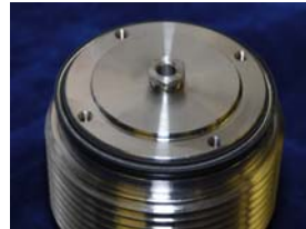
Cup seal fits onto cover. 100mL #7521, 300mL #7525, 500mL/1L #7318
