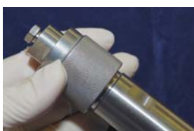
Closure nut finger tightens onto end of vessel.
