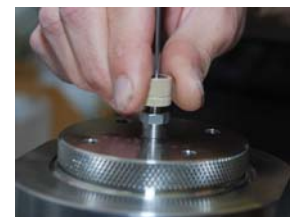
Vessel connector attaches to closure nut.
